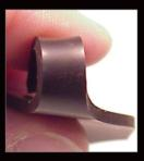
The fluorocarbon elastomer specimen exposed to Mobil Jet Oil 387 is pliable and shows no cracks.
