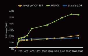
Mobil Jet Oil 387 provides superb compatibility and prolonged seal life. Compared to the competitive oil tested, Mobil Jet Oil 387 offers improved protection against oil leaks.
