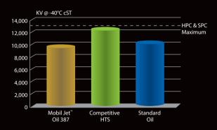
Mobil Jet Oil 387 has better low-temperature fluidity compared to competitive HTS oil and standard oil, making it more suitable for APU operation on ETOPS aircraft.
