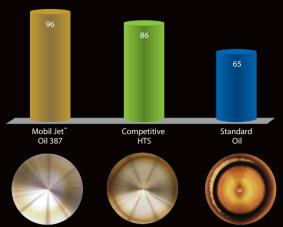
The Thin Film Oxidation test\* predicts oil's ability to resist deposit formation when subjected to extreme temperatures and oxidation.
