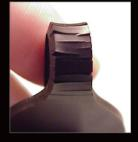
The fluorocarbon elastomer specimen exposed to competitive HTS oil is brittle with visible cracks.
